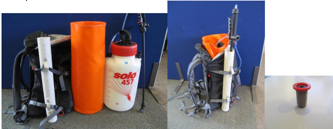
Figure 1: The components of a 7.5 litre backpack spraying system for applying a basal bark treatment to invasive trees. Note non-drip valve for spray nozzle. (Photos: Peter Willemse).
